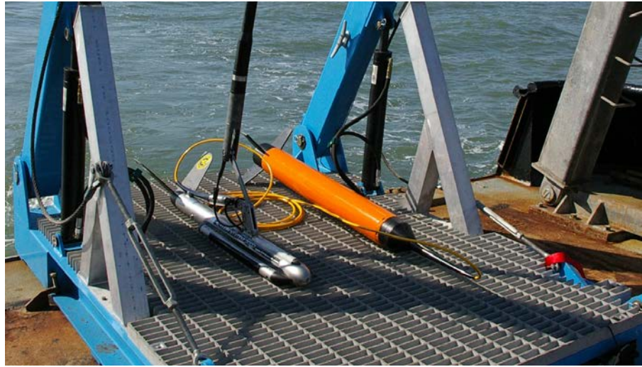
Image 1: SeaSpy Magnetometer and Klein 3000 Towfish Ready for deployment
